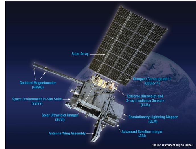
Figure 2. GOES-R Series satellites are composed of 6 (7 on GOES-U) instruments, and powered by a solar panel array.
